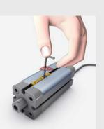
Stable fitting The sensor is inserted in the groove and then tightened by a quarter turn with flat-tip screwdriver or a 1.5 mm Allen wrench. The screw is made of tool steel alloy to ensure stable fitting.
