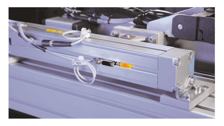
You can now query the piston position on standard pneumatic cylinders very comfortable with a single sensor type. The new magnetic field sensors BIM-UNT, BIM-UNTK and BIM-UNR by Turck not only support efficient standardization, they also offer more leeway for optimization in terms of construction, purchase, production, operation and service. Use the unique performance spectrum of these sensors and reduce your application costs effectively
